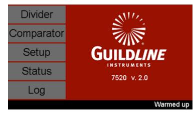
analogue circuits that are part of the voltage divider network and self-alignment circuitry. This high isolation ensures no offsets will be present in measurements due to leakage or noise from the rest of the circuitry inside the 7520. An easy to use Operating Menu is provided as per the screen image to the left. An operator has five selections from the Main Menu.
