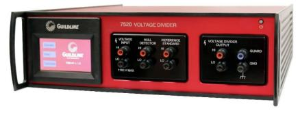
Special care has been taken to minimize thermal offsets and noise during use, and during the 7520 self-alignment/selfcalibration. The voltage reference, resistive voltage divider networks, and optical null detector are all inside a thermally regulated and EMI shielded chamber. The ultra-low thermal switches used are high isolation relays. In addition, the use
